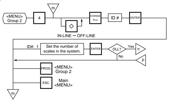
**NOTES:** 1. Before starting the above procedure, press the  $\Diamond$  key and enter IN-LINE mode.
